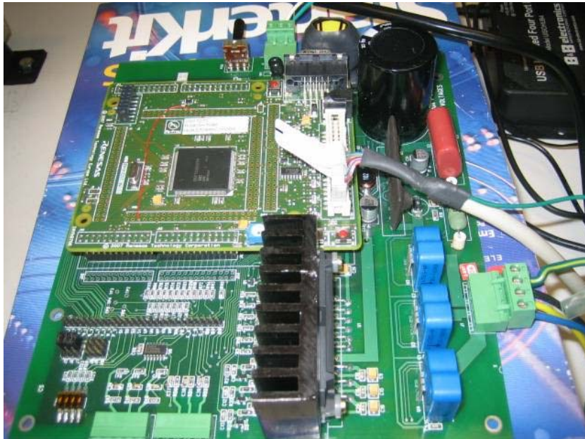
Fig. 6 Sensorless vector control implementation platform with current sensors from LEM USA.
